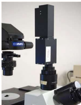
Attaching to camera port above eye-piece
